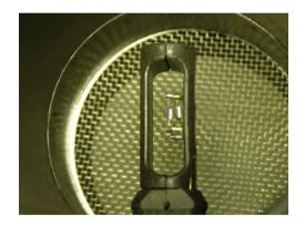
Source Z32 MAFs from reputable dealers. Counterfeits are plenty on the internet can have original looking stickers, part numbers but the inside sensor should be small wax coated bead as per the image on the left. A bad MAF results in incorrect airflow measurements and tuning problems!
